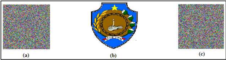
Figure 6. Key sensitivity analysis. (a) encrypted image (cipher-image) using key "abcdefghijklmnopq", (b) decrypted image using correct key "abcdefghijklmnopq", (c) decrypted image using wrong key "abcdefghijklmnopr".
